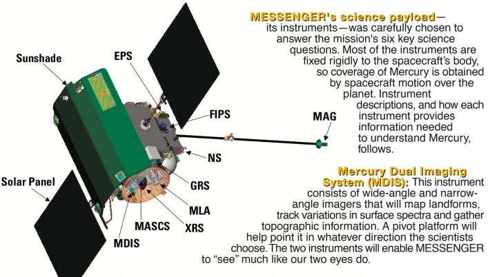
Gamma-Ray and Neutron Spectrometer (GRNS): This instrument will detect gamma rays and neutrons that are emitted by radioactive elements on Mercury's surface or by surface elements that have been stimulated by cosmic rays. It will be used to map the relative abundances of different elements and will help to determine if there is ice at Mercury's poles, which are never exposed to direct sunlight.
